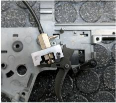
3: Temporarily install the other half of the gearbox shell and feel if there is any free play between the trigger and the plunger on the 3-way valve. There should be at least a slight gap and therefore a small amount of free play, between the trigger and the plunger of the 3-way valve.
