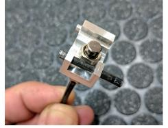
2:Install the 3-way mount assembly into the gearbox shell by inserting the body pin into the body pin hole and the stub pin on the 3-way mount into the hole to the rear of the body pin hole. Then install the trigger **without** the trigger spring.
